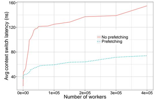
Figure 5: Average context switch time with and without prefetching.
